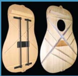
If you like the idea of the suspended bracing system but hanker after a more conservative-looking instrument, Boulder Creek's 'Stage & Studio' series should fit the bill. These guitars feature a standard soundhole design but still get the bracing that features on the Solitaire.
